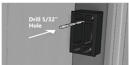
3 Attach 1/4 inch drill bit into drill and drill through 1/4 inch hole in drill block.
