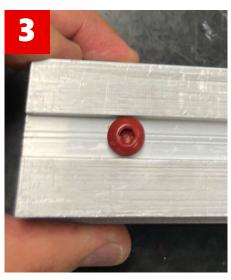
Locate the two red shipping screws on each end of Katy Bar in bottom rail.
