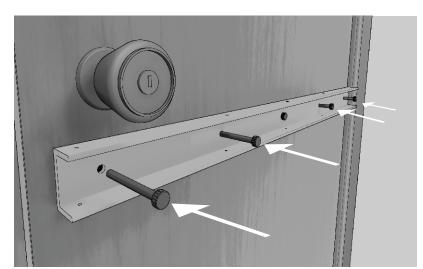
Find center of each remaining holes in Door Rail, mark and punch to create indent. Repeat the process of 5/32", then 1/4" hole with Drill Block for the remaining holes checking level and hand snug 1/4"-20 SS bolt & nut as each hole is completed.
