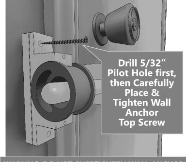
WARNNG: DO NOT OVERTIGHTEN WALL ANCHOR FRAMING SCREWS & CRUSH WALLBOARD
