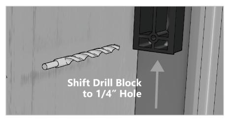
4 Align 1/4 inch drill bit with 5/32 inch hole and with drill block flat against door frame, drill 1/4 inch hole in frame. Remove drill bit
