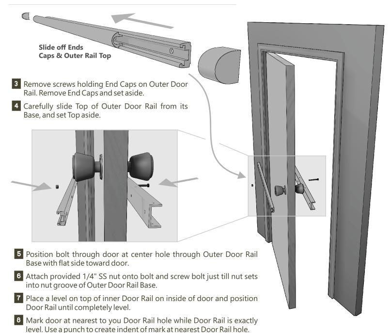
! It is critical to drill holes through casing straight & level in order for bolts to move freely into frame.
