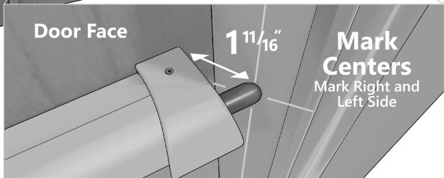
2 At the marked locations on frame, use the hammer and punch to create indent at exact center for drilling
