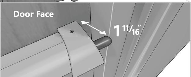
3 The distance from face of door to the center of lock bolt is 1 11/16 inches. Doorframe is smooth on both sides and will not interfere with lock bolt installation through frame.
