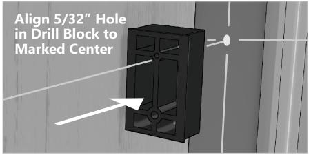
2 Attach 5/32 inch drill bit into drill and drill through 5/32 inch hole in drill block. Align 5/32 inch drill bit with punch indent and with drill block flat against door frame, drill 5/32 inch hole into frame. Remove drill bit.
