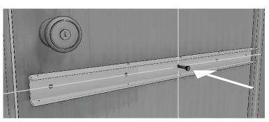
Position bolt at center hole through Outer Door Rail Seal with flat portion of seal toward door. Open door midway to make installation easier.
