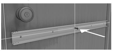
Use punch to indent holes on door. Repeat marking each remaining hole. Starter holes are often all that is needed for many doors. If you need to drill a complete hole, do so with the taped drill bit for each door rail screw.
