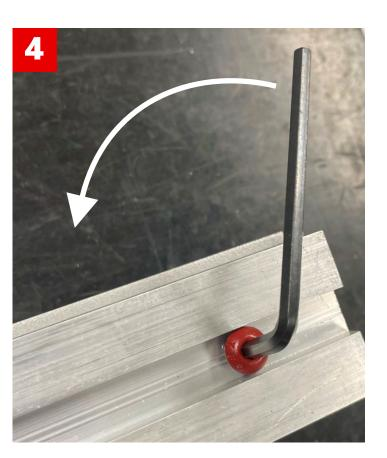
Use provided wrench to remove the shipping screws and discard.
