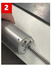
Using screwdriver, pry upward to separate the Katy Bar from the door rail.
