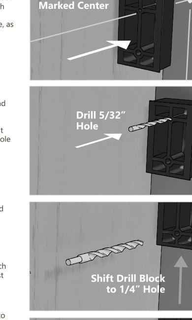
Align 5/32" Hole in Drill <u>Block to</u>
