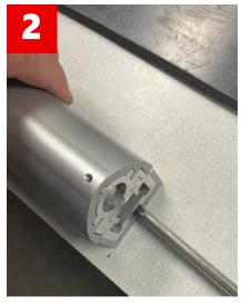
Using screwdriver, pry upward to separate the Katy Bar from the door rail.
