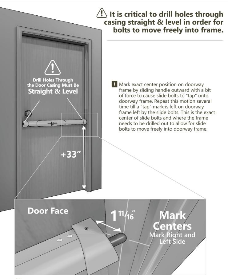
2 At the marked locations on frame, use the hammer and punch to create indent at exact center for drilling
