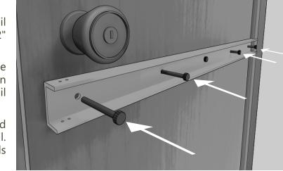
9 Find center of each remaining holes in Door Rail, mark and punch to create indent. Repeat the process of 5/32", then 1/4" hole with Drill Block for the remaining holes checking level and hand snug 1/4"-20 SS bolt & nut as each hole is completed.
