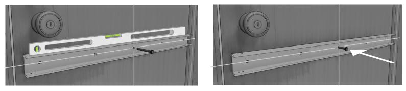
2 Position bolt at center hole through Outer Door Rail Seal with flat portion of seal toward door. Open door midway to make installation easier.
